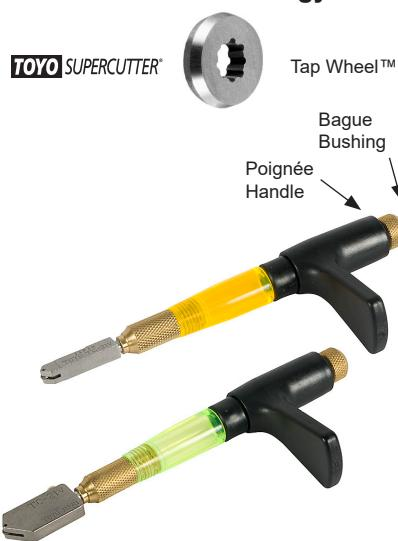
Developed for thick glass (10-19 mm), it has been adapted for cutting 2-9 mm glass, including art glass. The TAP Wheel™ has a unique axle bore with eight microscopic cams creating eight taps per revolution of the wheel. The cams improve axle lubrication, reduce rolling friction and allow the score to be driven deeper into the glass with less pressure. The result is a longer wheel life and a clean, consistent score.
